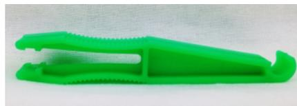
Figure 1 - 3AG Fuse Puller
